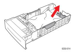
**3.** Verify that the paper is loaded correctly in the tray and the guides are set flush against the paper.
