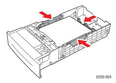
**4.** Remove jammed paper from inside the printer tray slot. Verify that all scraps of paper are removed.
